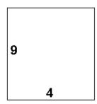
surface area = 2(length x height) + 2(height x width) + 2(width x length)
